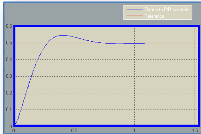
Figure (6.2): Step response of maglev CE152 with PID controller
